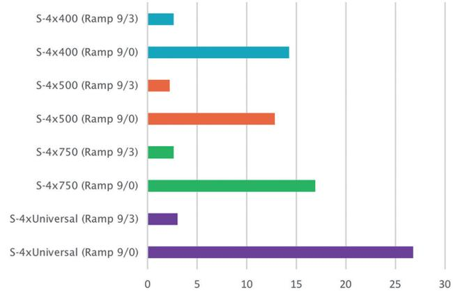
**Figure 5:** Brake times determined for the new Eppendorf Multipurpose Centrifuge 5910 Ri, used in combination with different swing-out rotors at ramp settings of either 9/0 or 9/3, respectively (rotors were fully loaded; the brake times decrease with decreasing load).
