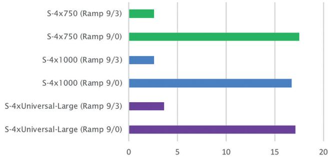
**Figure 4:** Brake times determined for the new Eppendorf Multipurpose Centrifuge 5920 R, used in combination with different swing-out rotors at ramp settings of either 9/0 or 9/3, respectively (rotors were fully loaded; the brake times decrease with decreasing load).
