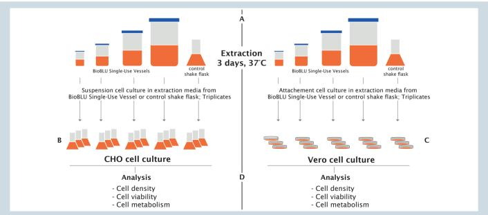
**Fig. 2:** Experimental setup. **A:** Extraction with medium. **B:** CHO-cell culture in extraction media. **C:** Vero cell culture in extraction media. **D:** Analysis of cell density, viability, and metabolism.
