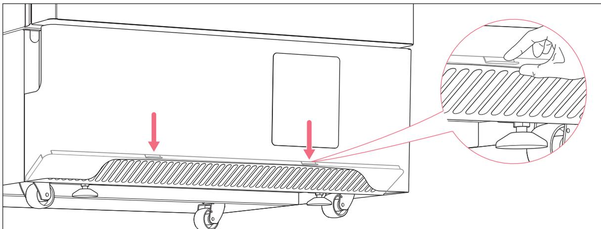
Fig. 9-1: Folding down the air intake grille
