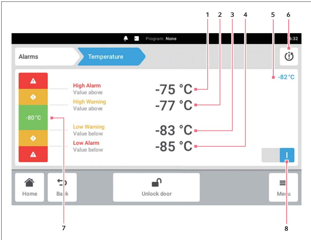
Fig. 7-3: Overview of the *Temperature* hazard message
