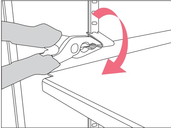
1. Use pliers to hold the lower part of the assembly clip.
