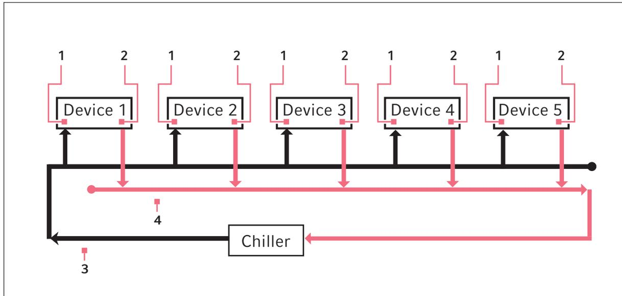
Fig. 4-4: Connection principle
