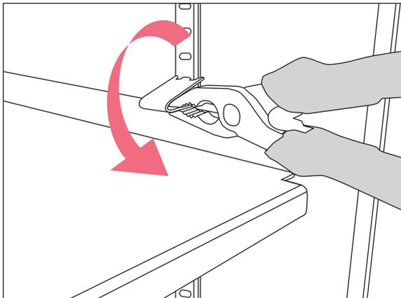
3. Carefully turn the pliers counter-clockwise for removing the assembly clips on the right side.
