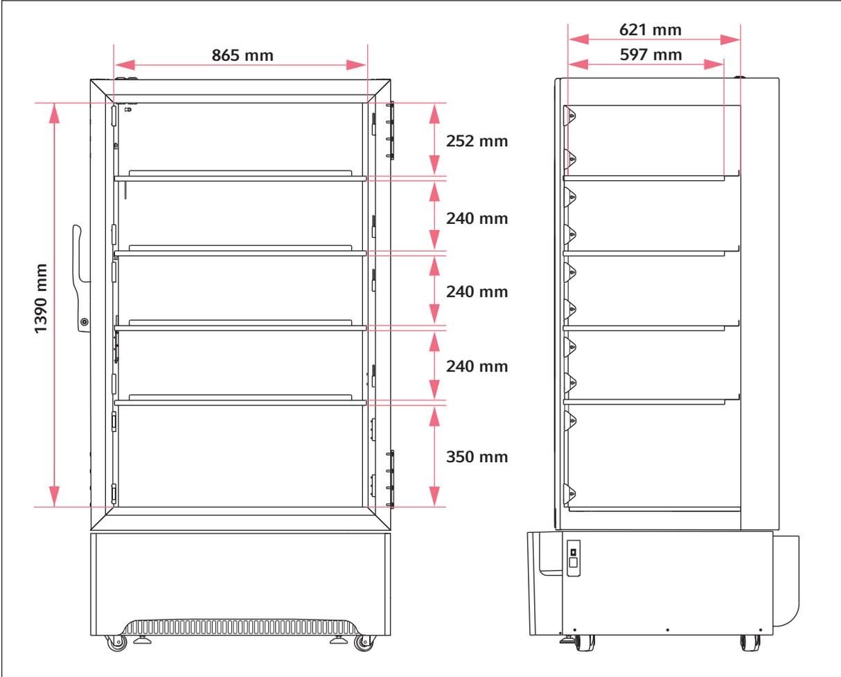
Fig. 12-2: Internal dimensions for devices with 5 inner compartments
