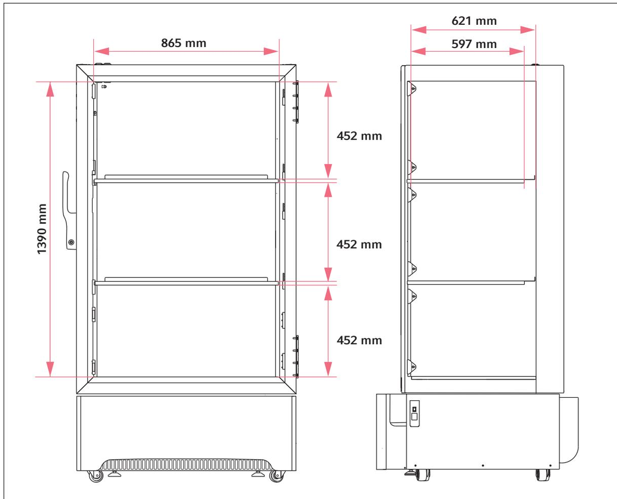
Fig. 12-3: Internal dimensions for devices with 3 inner compartments
