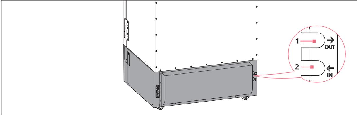
Fig. 3-4: Connections for the cooling water supply
