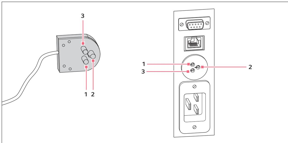
Fig. 4-5: Plug and remote alarm interface
